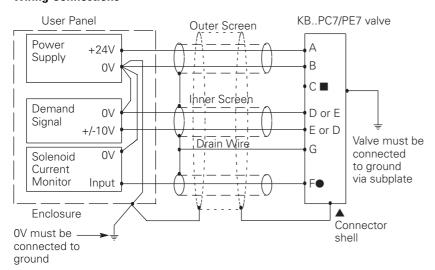
■ Pin C may be connected to ground or left unconnected.
